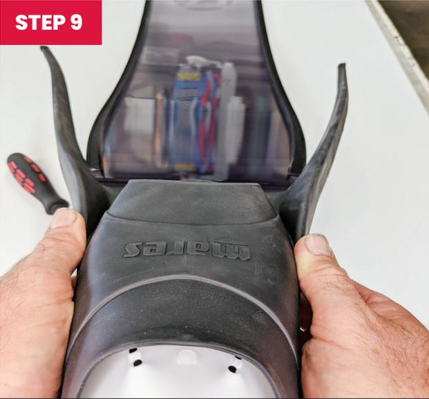
Sight along the top of the fin and ensure the blades are aligned with the pocket.
