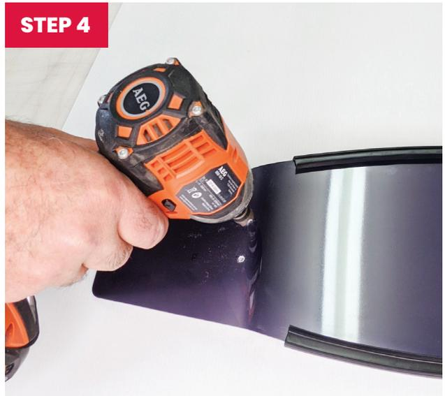
Using a countersink drill-bit, remove any sharp edges or burrs from the holes.
