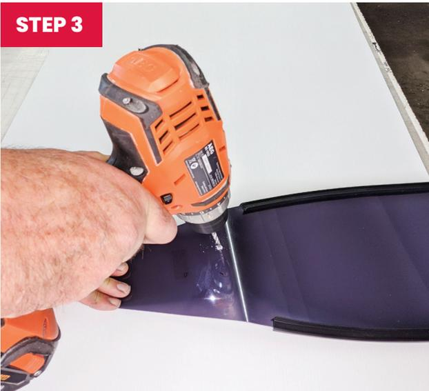
Drill 4mm holes - using light pressure in the centre of the permanent marker dots from step 3.
