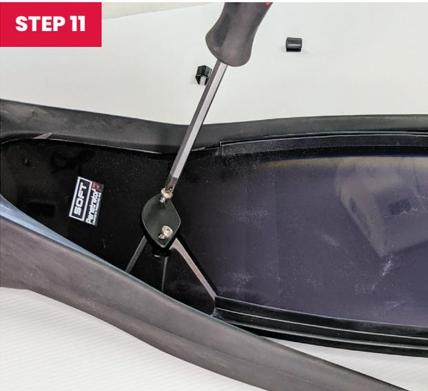
Fully tighten the fixing kit screws with the plate positioned as shown. Do not overtighten.
