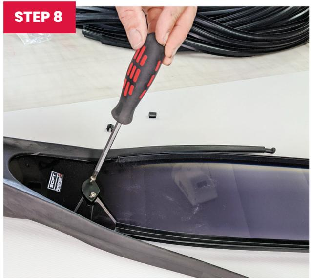
Place the bottom plate and screws in position and tighten screws half way only.
