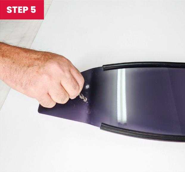
A larger diameter drill bit can also be used to remove sharp edges or burrs (by hand only).
